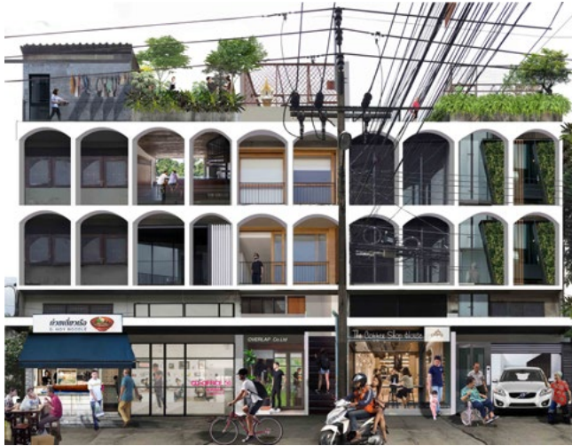
Fig.2: A possible street elevation of a row of shophouses in Bangkok once the owners have adopted and applied a design guideline for improvement of modern shophouses built during the 1960s and 1970s according to their own needs while conforming to regulations and achieving a certain level of unity in design, thanks to the maintenance of standardized concrete screens.
